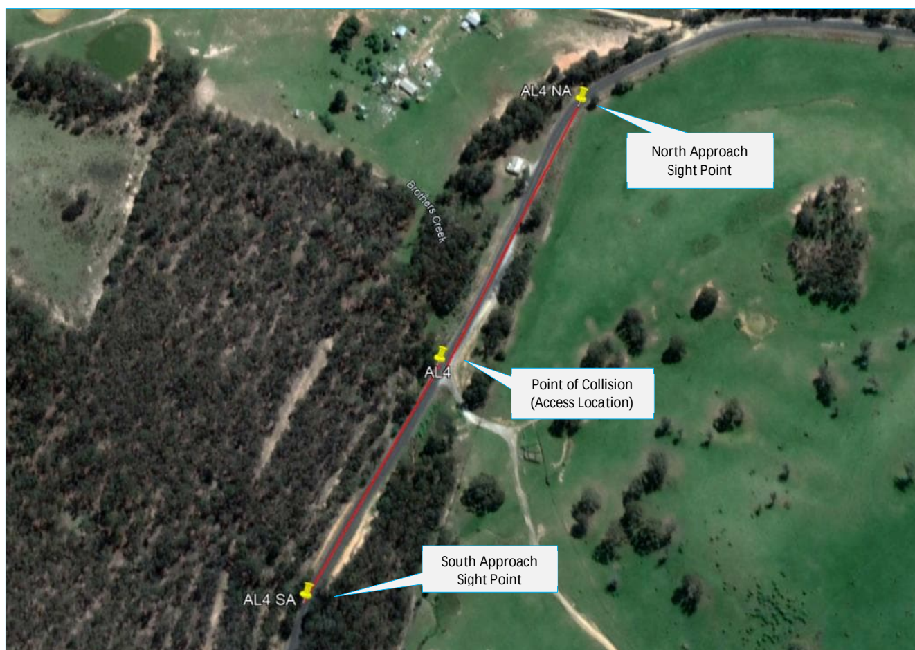
Figure 20 Access Location 4 and Relevant Sight Distances
