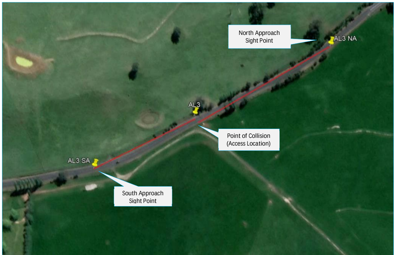
Figure 18 Access Location 3 and Relevant Sight Distances
