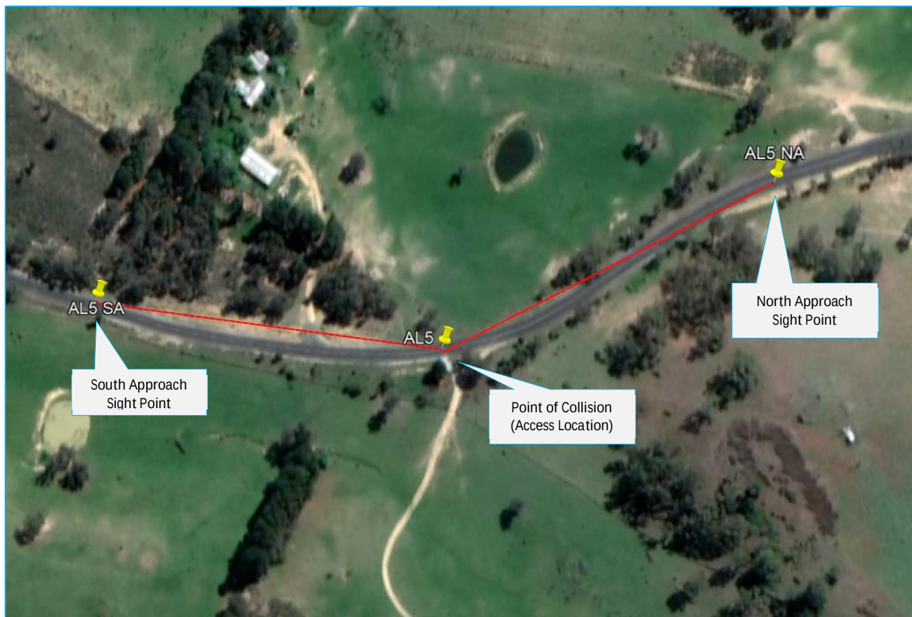
Figure 22 Access Location 5 and Relevant Sight Distances
